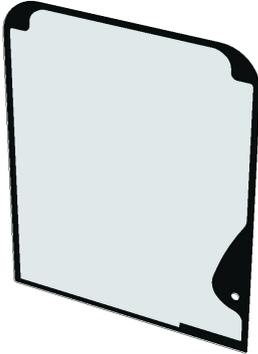
Hammerglass screen to replace the original screen. With factory mounted ScreenSaver protective film. To be glue mounted as the original screen. NOTE! Use elastic glue! Do NOT use ordinary car glass glue. The film can be replaced when scratched or damaged.
